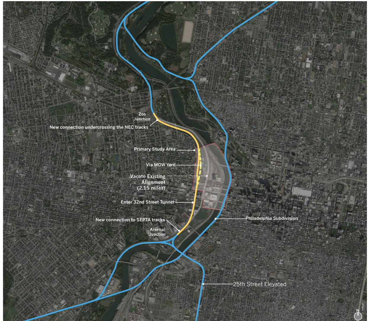
FIGURE C.4 ALTERNATIVE 4 - SHIFT ALIGNMENT WEST VIA POWELTON YARD OR MAINTENANCE OF WAY YARD Credit: SOM in association with Parsons Brinckerhoff, OLIN and HR&A
